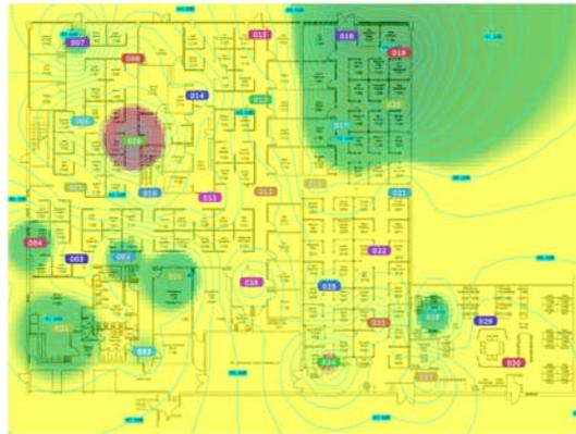
unintentional radiator. The operator then selected, by drag and drop, the second observed frequency to render a new heat map display specific to the center frequency and utilized the Reference Level Off-Set (RLO)<sup>™</sup> to better characterize
