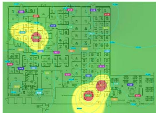
frequency, two (2) additional workstations at < 023 > and < 024 > were identified as potential unintentional radiators at 389.7200 MHz, not identified as emitters with
