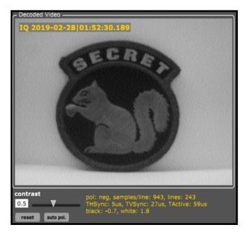
The above window represents actual video content captured and played back from an Kestrel IQ (KIQ) <sup>TM</sup> file utilizing the Kestrel TSCM <sup>®</sup> Professional Software without the need of a connected radio to render video and audio playback.
