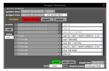
Once the operator-defined event scheduler is programmed, either manually, or via a standard CSV master file, the operator can press the "resume schedule" button to allow full software automation for unattended deployment of the platform.
